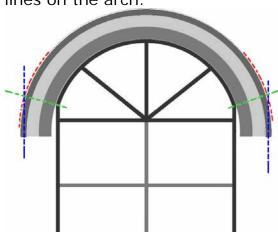
5. Place the trims back on the sides of the window and mark the join lines on the trims.
