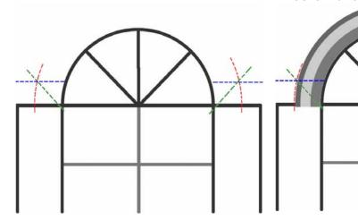
5. Place the trims back on the sides of the window and mark the join lines on the trims.
