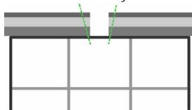
3. Glue the keystone, and the two half trims in place. Use FLEXOCOAT in the joins.
