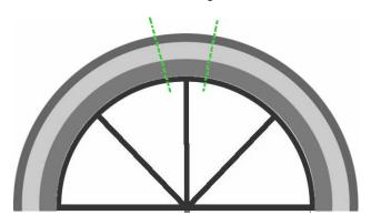
3. Glue the keystone, and the two half arches in place. Use FLEXOCOAT in the joins.
